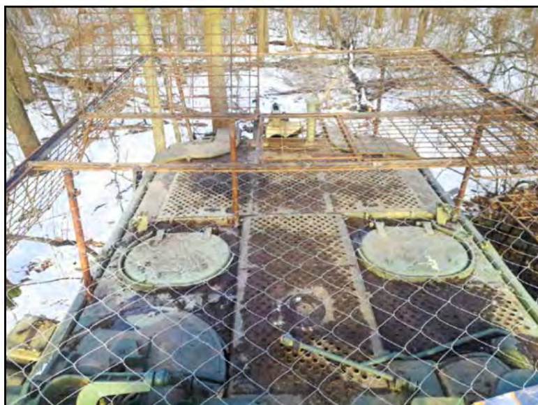
Fig. 8. Protection of armored vehicles from chain-link mesh against drops and simple FPV
