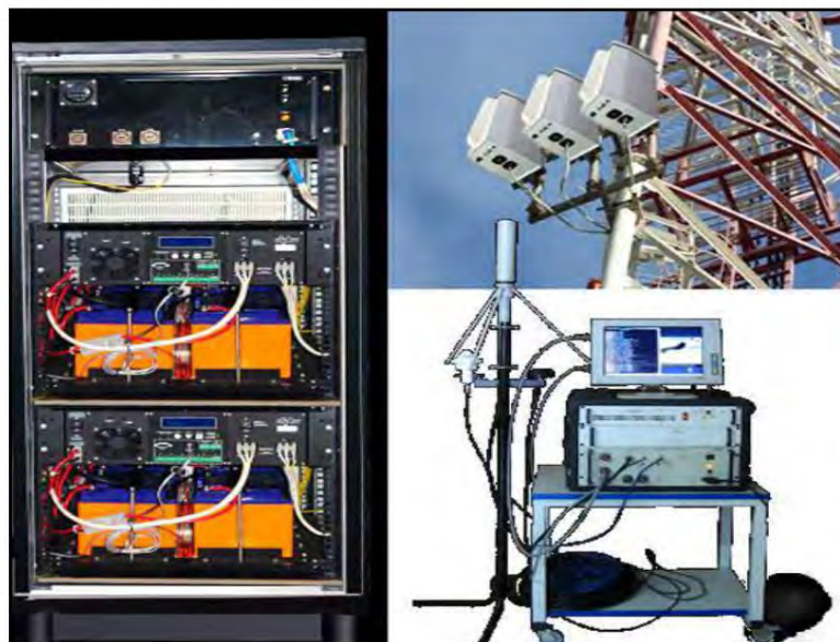
Fig. 15. Facilities of the Pole-21 complex: rack with equipment (left), antenna modules (top right) and control panel
