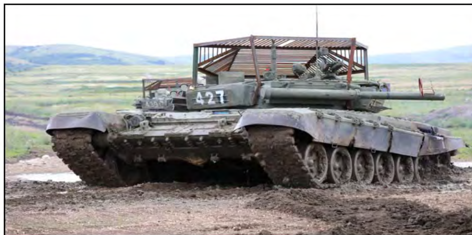
Fig. 7. Tank with a protective steel visor
