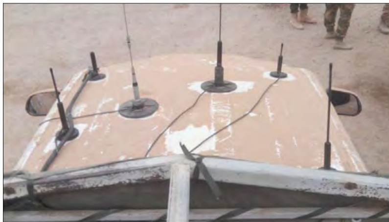
Fig. 12. Placement of the "Lesochok" jamming station on the hood of a car
