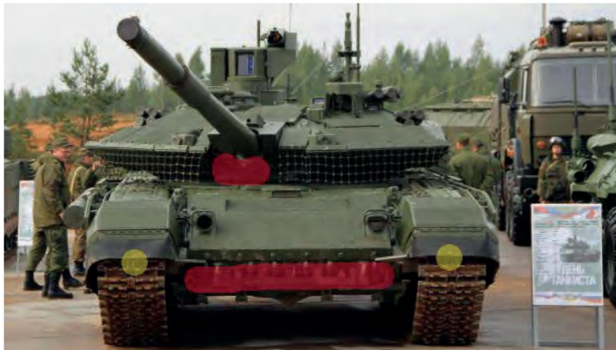
Figure 1.5.2 – T-90M “Breakthrough”, front view and its areas of damage by non-tandem grenades
