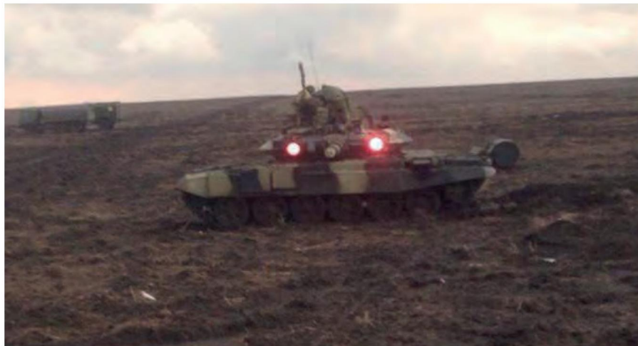
Figure 1.4.1 – T-90A. The Shtora complex is turned on and because of it the tank unmasks itself very well even during the day.
