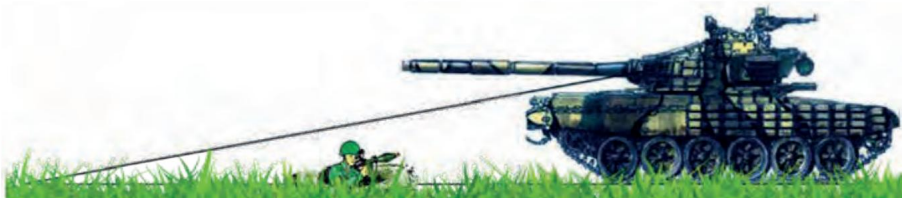
Figure 2.1.2 – Dead zone for the rear weapons of the T-72, T-80, T-90 tank – 37 m
