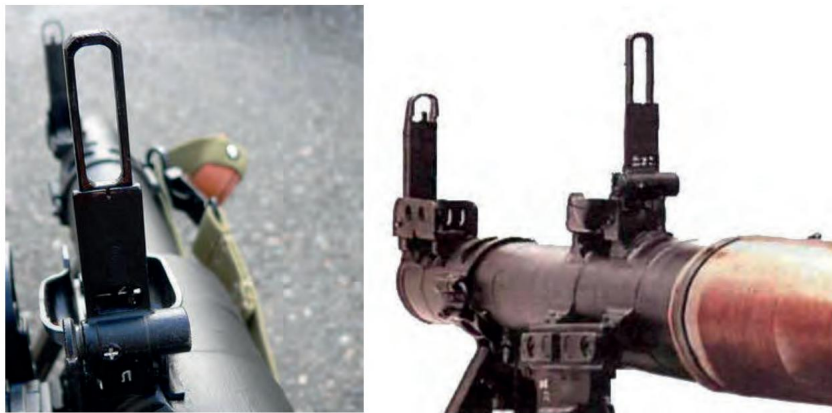
Figure 3.1.20 – RPG-7 mechanical sight
