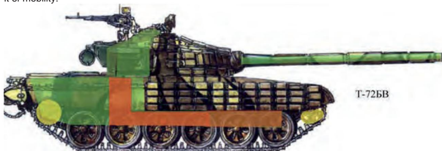
Figure 1.1.1 – Vulnerable zones of T-72BV and T-80BV with single-action grenades when fired at the side
