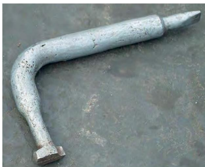
Figure 2.1.5 – "Tank key" or as it is also called – turret key
