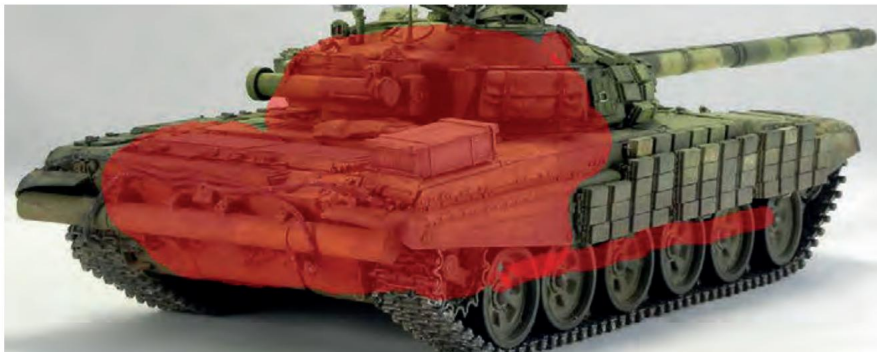
Figure 1.1.3 – Vulnerable zones of T-72BV, T-80BV tanks from single-action grenades when fired from behind
