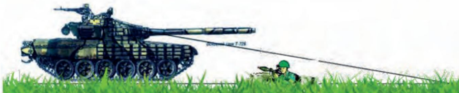
Figure 2.1.1 – Dead zone for weapons of T-72, T-80, T-90 tanks in front – 20 m
