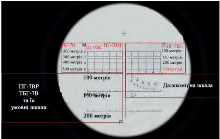
Figure 3.1.17 – Real and conditional aiming scales for different types of grenades
