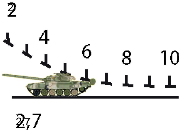
Figure 3.1.18 – Determining the distance using the rangefinder scale of the grenade launcher optical sight (distance to the target is 500 m, if the target is 2.7 m high)
