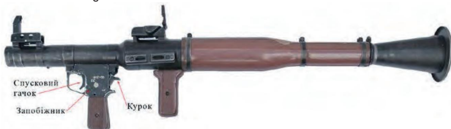
Figure 3.1.14 – Location of the safety, hammer and trigger in the RPG-7 of all modifications, including the RPG-M7 produced in Ukraine
