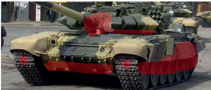
Figure 1.2.2 – Tanks of the T-72, T-90, T-80U type with the Kontakt-5 DZ, the affected areas
