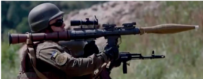
Figure 3.1.3 – The RPG-7, manufactured in the USA and supplied to Ukraine, has modern improvements in the form of Picatinny rails for mounting optics, and the name "PSRL-1"
