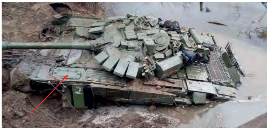
Figure 2.1.6 – T-72B3 tank; location of the spare parts box with the tank key (red arrow)
