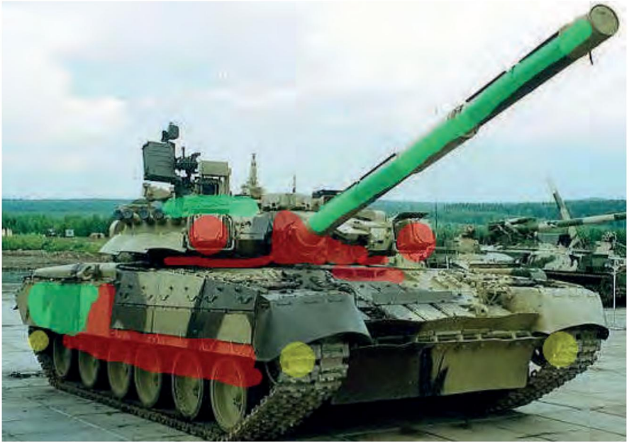
Figure 1.4.2 – T-80UA. Damage from non-tandem grenades, front. To the right and left of the gun are two “box-shaped” blocks of the “Shtora-1” complex. The complex is turned off
