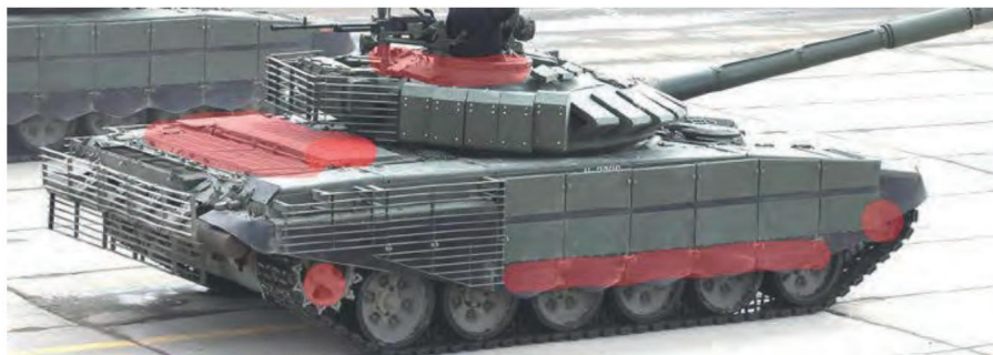
Figure 1.3.1 – T-72B3M and T-80BVM damaged by grenades non-tandem action, side and rear
