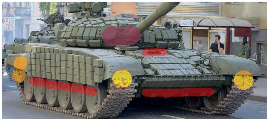
Figure 1.1.2 – Vulnerable zones of T-72BV, T-80BV during frontal fire
