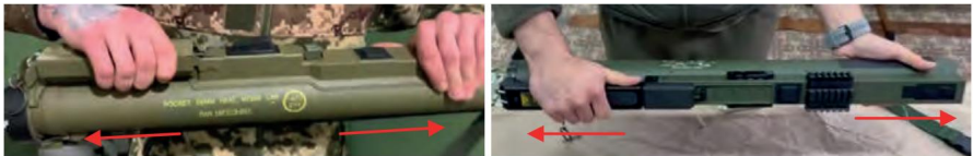
Figure 3.12.4 – Stretching of A6 (left) and EC Mk.I (right) pipes; arrows – direction of movement
