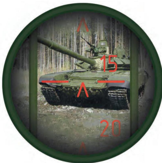
Figure 3.2.3 – Visibility through the sight of the RPG-18 model of 1972. The distance to the T-72B3 tank is 150 m.
