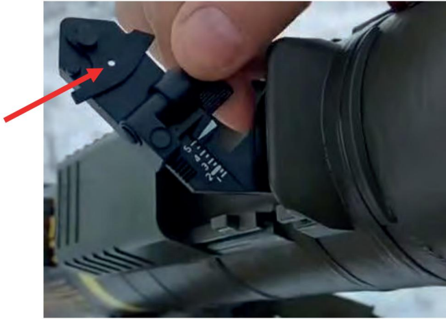
Figure 3.5.6 – Sight in combat position. The arrow indicates the diopter.
