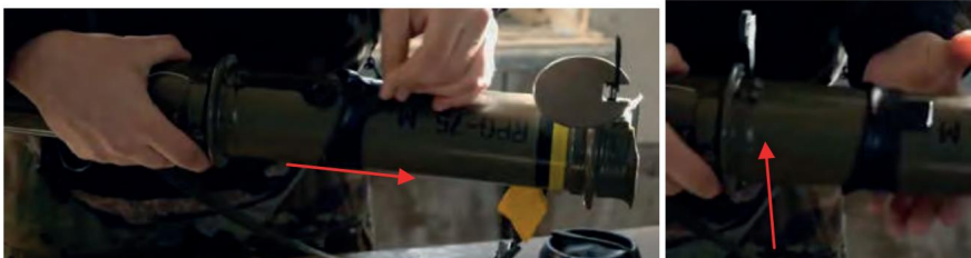
Figure 3.9.3 – Releasing the sighting bar
