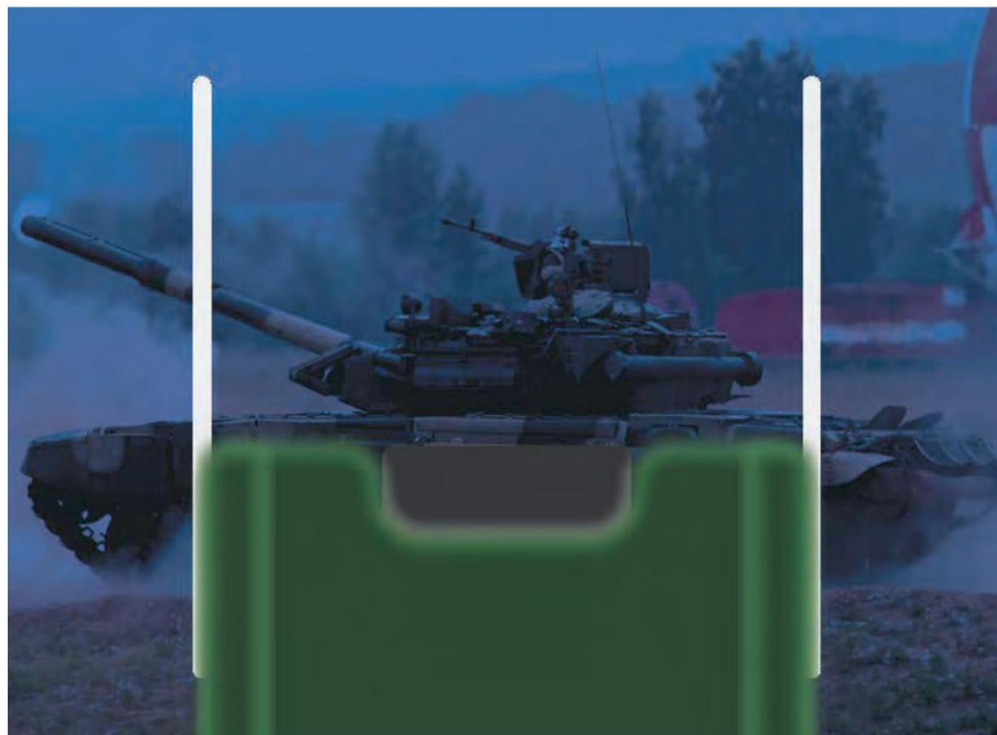
Figure 3.3.4 – Night visibility through the RPG-22 night sight, the distance to the T-90 tank is 100 m. Vertical white lines – diopter rack mounting
