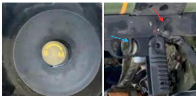
Figure 3.11.3 – Main part of the boom (left). On the right – fuse (red arrow) and trigger (blue arrow)
