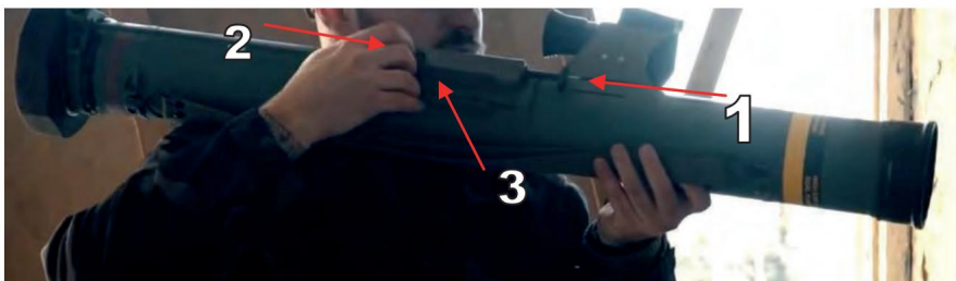
Figure 3.10.5 – 1. Cocking lever; 2. Safety catch; 3. Firing button
