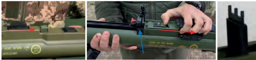
Figure 3.12.5 – Moving the safety catch – red arrows and direction of movement A6 (left) and EC Mk.I (center); Sight – blue arrow; Front sight (right)
