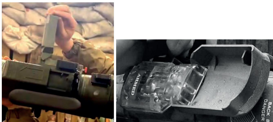
Figure 3.6.8 – Deploying the firing mechanism safety cover
