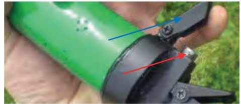
Figure 3.8.6 – Blue arrow – safety catch; red arrow – firing button
