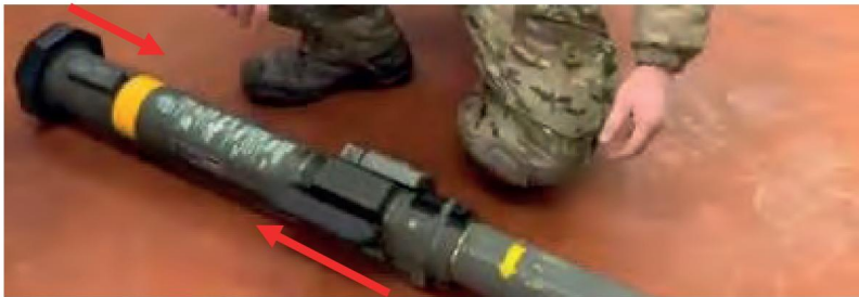
Figure 3.6.5 – Unlocking and deploying the shoulder stop
