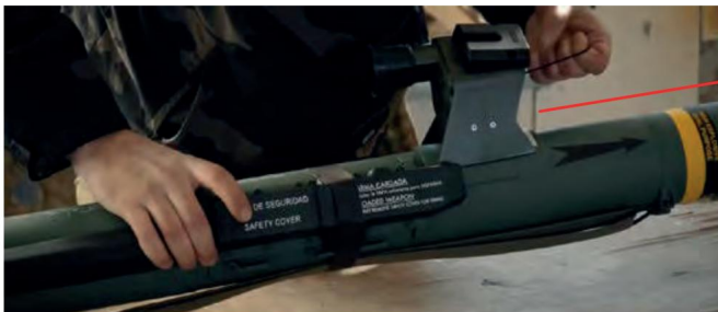
Figure 3.10.3 – Removing the cover from the scope – pull the string
