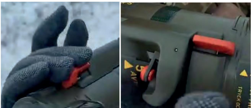
Figure 3.5.8 – Left – the safety is pushed up; Right – Location of the trigger button behind the safety on the RPG. The yellow arrows show the direction of movement of the push
