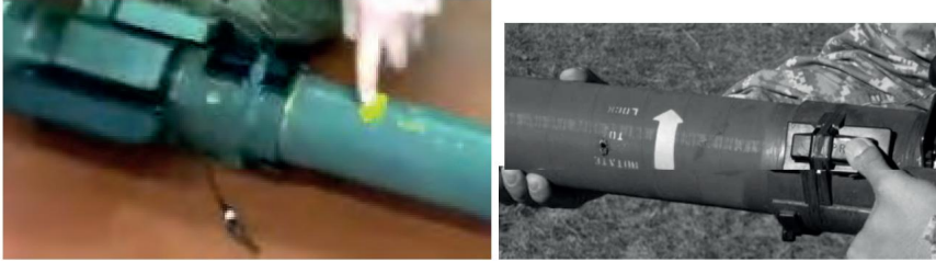
Figure 3.6.4 – Pulling and locking the pipe
