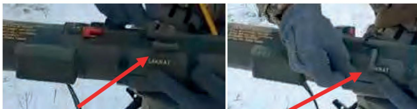
Figure 3.5.3 – Left – bolt in stowed position; Right – bolt in firing position
