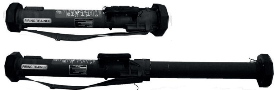
Figure 3.6.1 – M141 in stowed (top) and combat positions
