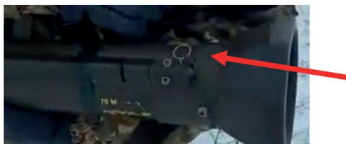
Figure 3.5.2 – Transport ring, marked with a red arrow
