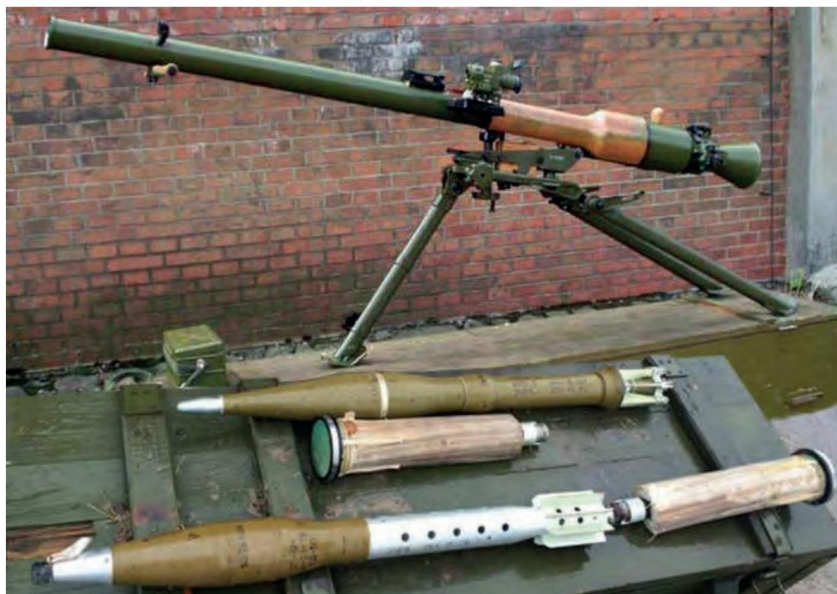
Figure 3.13.1 – SPG-9 on bipod with PG-9VS grenades (top) and OG-9V prepared for firing (bottom)
