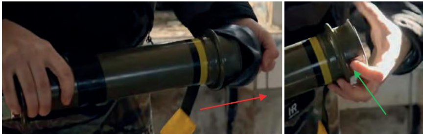
Figure 3.9.2 – Removing the rubber cover (left), red arrow – direction of movement; Front sight button (right), green arrow direction of movement when pressed
