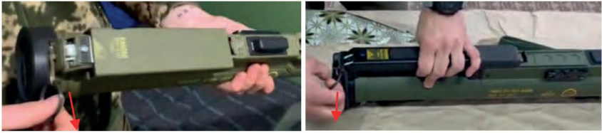
Figure 3.12.3 – Pulling out A6 checks (left) and EC Mk.I (right), arrows – direction of movement
