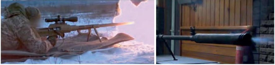
Figure 4.1.3 – Flame with muzzle brake (left), and with silencer
