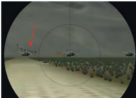
Figure 5.1.11 – Reticle of the ATGM “Fagot” / “Konkurs”. The red arrow is a distance mark. According to the figure, the T-72B3M tank is 1500 m away.
