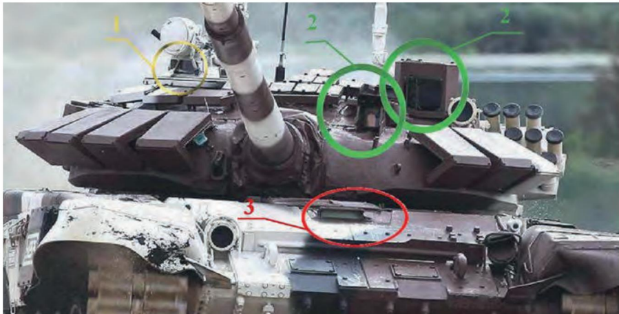
Figure 4.1.15 – Locations of T-72 observation and aiming devices vulnerable to AVG, the failure of which blinds the tank crew. The numbers indicate: 1 – commander's sight; 2 – gunner's sights; 3 – driver's triplex
