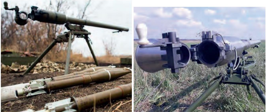
Figure 3.13.4 – SPG-9 “Kopyo” (left) and SPG-9AM “Lanceya” (right) with the bolt open and shots prepared
