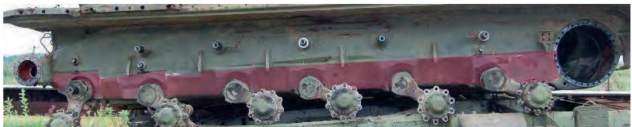
Figure 4.1.14 – As can be seen in the photo, the T-80U series tanks have a similar weakened, only 35 mm section with a camber of 100 (highlighted red), vulnerable to AVGP and RPG
