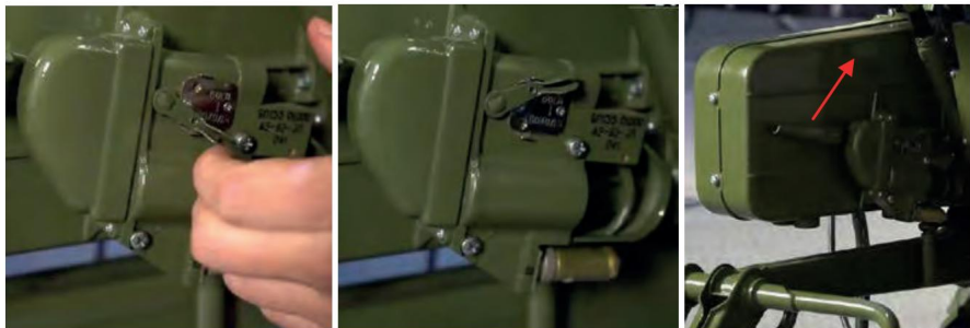
Figure 5.1.8 – From left to right: Safety catch in the stowed position; Safety catch in the firing position; Cocking the trigger mechanism, arrow – direction of movement
