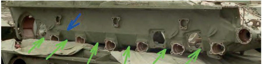
Figure 4.1.13 – The same 20 mm section of the side of the T-72/T-90 tanks – shown by green arrows, located below the weld of the upper side plate – marked by a blue arrow.
