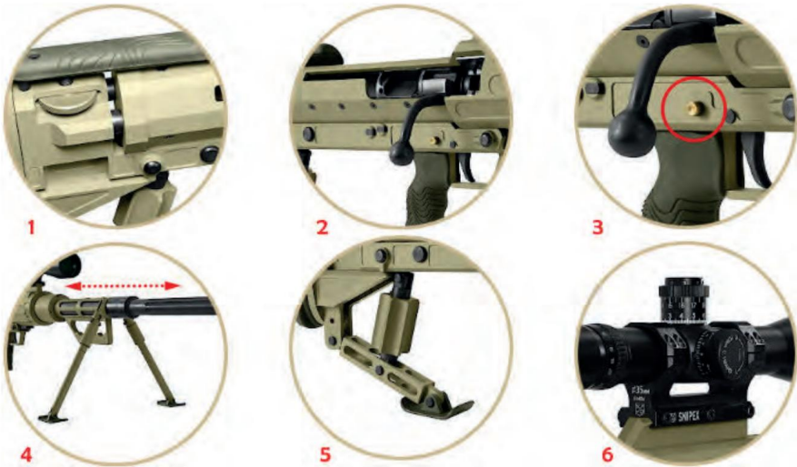
Figure 4.1.2 – Numbers indicate: 1 – Cheek rest; 2 – T-REX shutter; 3 – Safety catch (red circle); 4 – Folding bipod and easily removable barrel mount (red arrows – movement in the direction of assembly-disassembly); 5 – Adjustable rear support; 6 – Snipex JOVE 50 optical sight
