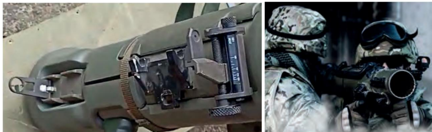
Figure 3.14.19 – Mechanical sight with front sight; on the right – aiming in Grg
