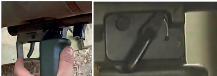
Figure 3.14.18 – Fuse on "F" – opening fire
