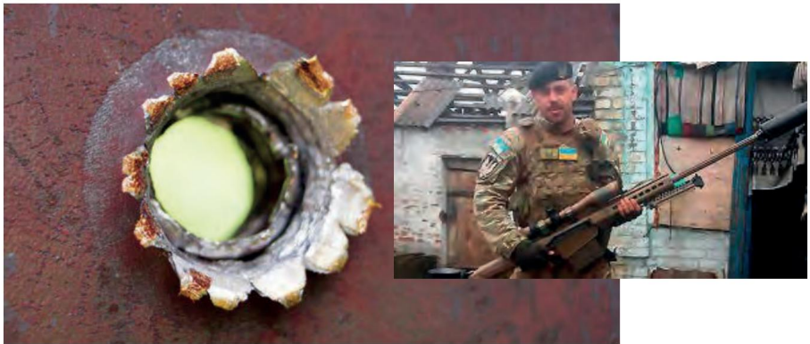
Figure 4.2.12 – The result of the .50 BMG cartridge on 12 mm thick armor plate at a distance of 400 m from a PGW LRT-3 rifle
