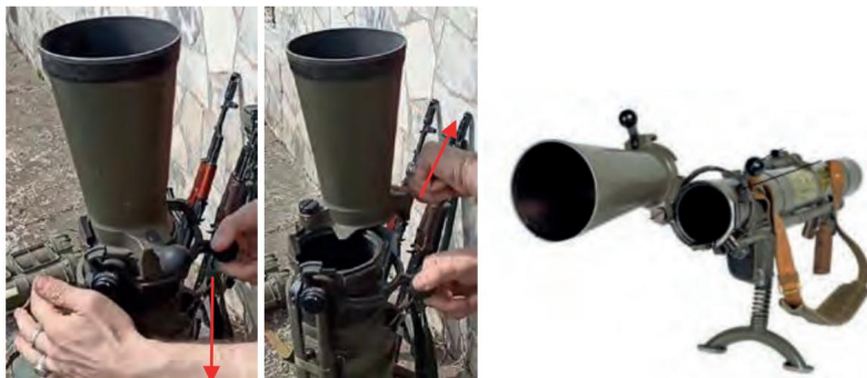
Figure 3.14.16 – Unscrewing the locking device (left) and opening the shutter (center); arrows – direction of movement
