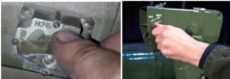
Figure 5.1.5 – Three shooting modes (left) and enabling the light filter
