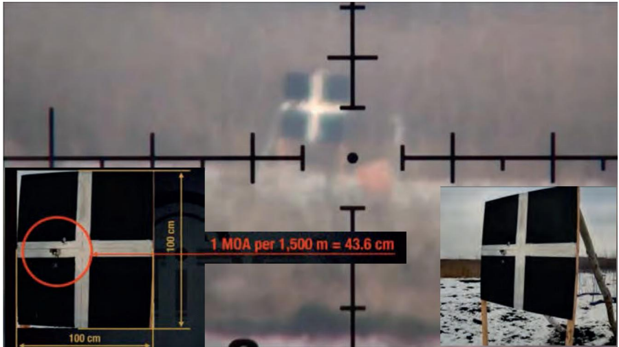
Figure 4.1.5 – Bias taken through the Snipex JOVE 50 sight at a target measuring 1.0x1.0 m, from a distance of 1500 meters; Insets show the results of hits
