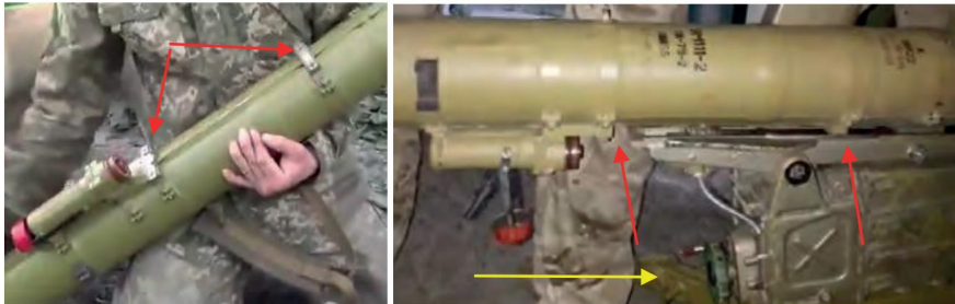
Figure 5.1.7 – Installing the rocket on the launcher. Red arrows – rocket container fasteners; Yellow arrow – direction of rocket movement along the runners
