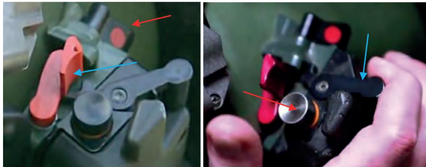
Figure 5.7.12 (left) – Red arrow: fuse; Blue arrow: safety bracket. Figure 5.7.13 (right) – Blue arrow – controller retention; Red arrow – start button
