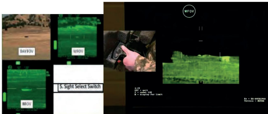
Figure 5.6.13 – Selecting the aiming mode
