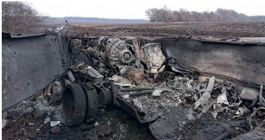
Figure 5.7.2 – Russian Army T-80BV tank, destroyed by the Kholodnyariv Infantry of the Armed Forces of Ukraine using the NLAW ATGM, no DZ helped – detonation of the BC, collapse of the turret, rupture of the hull completely. The thin, 20 mm, lower hull side sheet is clearly visible
