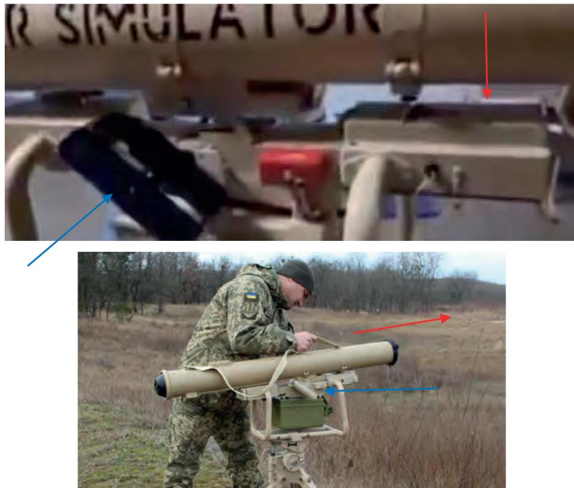
Figure 5.4.5 – Rocket installation. Red arrow – direction of movement when connecting; Blue arrow – launch handle
