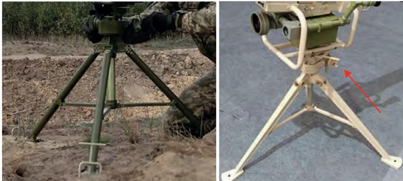
Figure 5.4.2 – Installing the tripod and trigger. Red arrow – mounting lever
