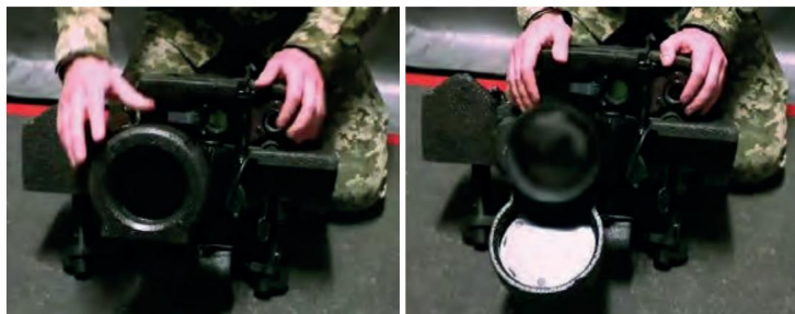
Figure 5.6.6 – Deploying the Sight's TPV
