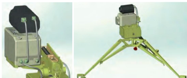
Figure 5.5.6 – Fastening the MSW and its cables
