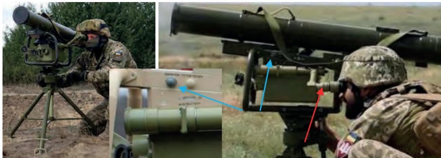
Figure 5.4.7 – Firing position. Red arrow – sight eyepiece; Blue arrow – complex activation button
