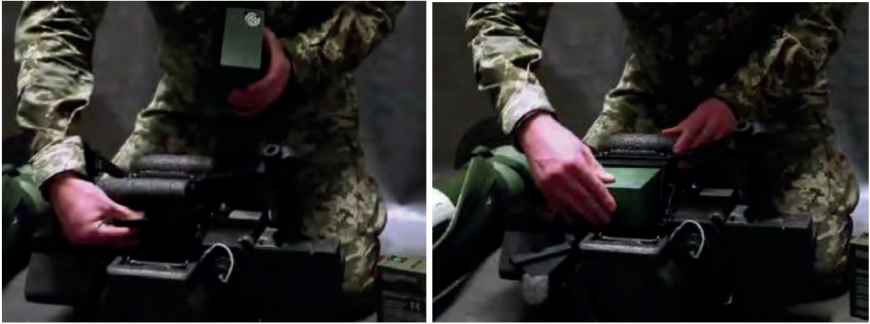
Figure 5.6.4 – Installing the power battery (enough for 2 starts)
