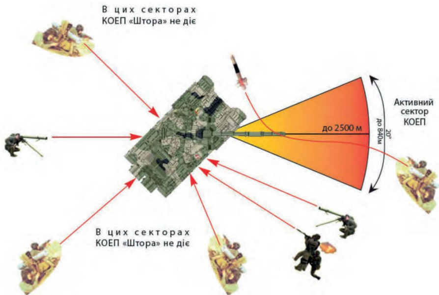
Item D.1 – Scheme of operation of the Shtora anti-tank missile defense system against tracer and coordinator
