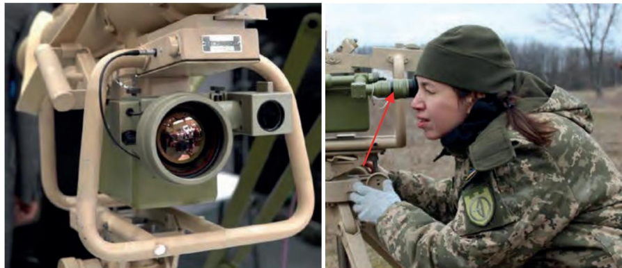
Figure 5.4.4 – Laser and optical channels; Arrow – sight eyepiece
