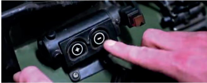
Figure 5.7.9 – Brightness control buttons
