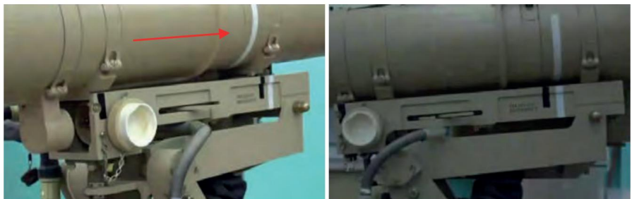
Figure 5.5.9 – Installation and fixation of the rocket, arrow – direction of movement
