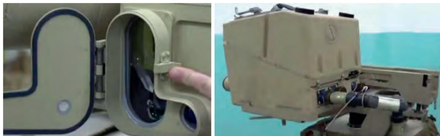
Figure 5.5.5 – Opening the window of the PN-I guidance device (left) and connecting the guidance device power cable
