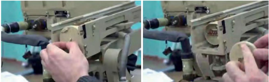
Figure 5.5.8 – Plug installed (left) and removed (right)
