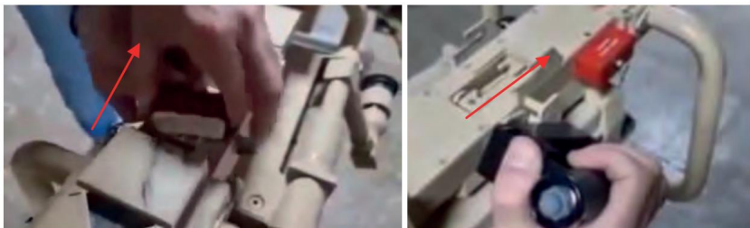
Figure 5.4.3 – Left – removing the plug; Right – the start handle, the plug has been moved in front of it; red arrow – the direction of movement of the start handle
