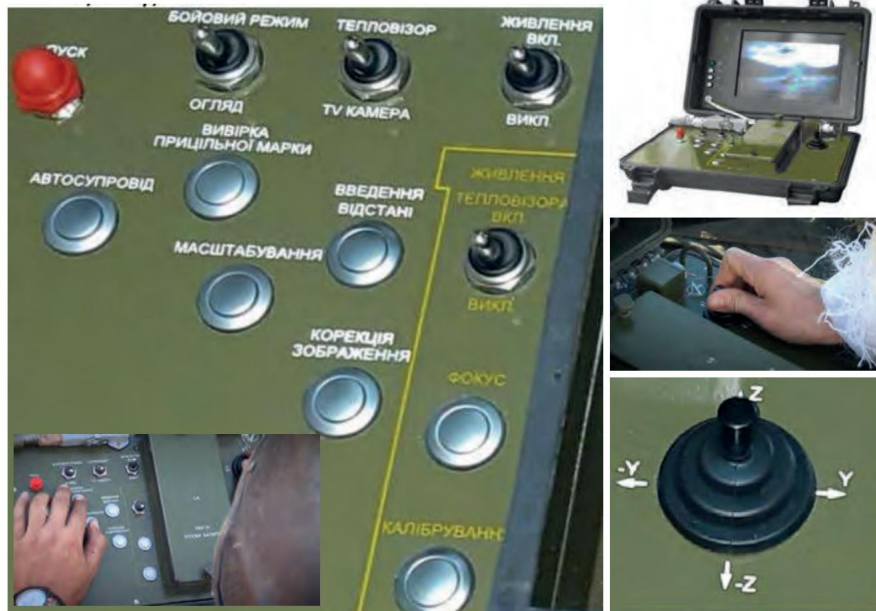
Figure 5.5.10 – Controls of the control panel, on the right – joystick for precise targeting of the missile
