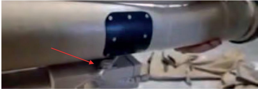
Figure 5.4.6 – Red arrow – Rear clamp lever and direction of movement
