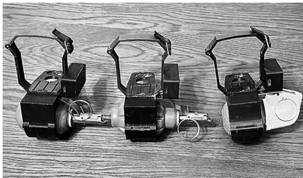
Dropping systems based on the interaction between the UAV's lighting and a photosensor, which initiates the drop by mechanically unlocking the lock that prevents the ammunition from falling
