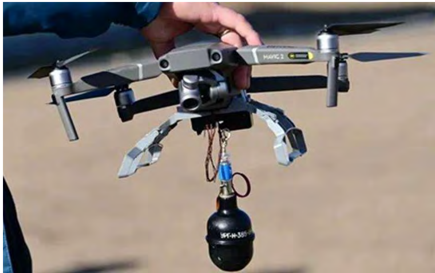
DJI Mavic 2 quadcopter with grenade launcher
