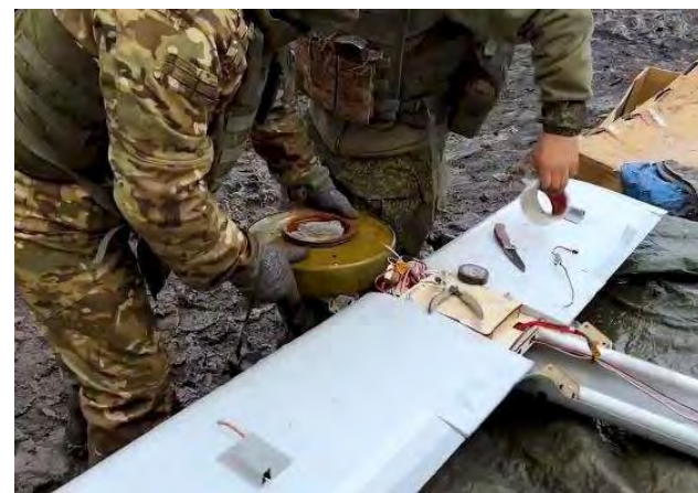
TM-62M mine prepared for use with UAVs Molniya
