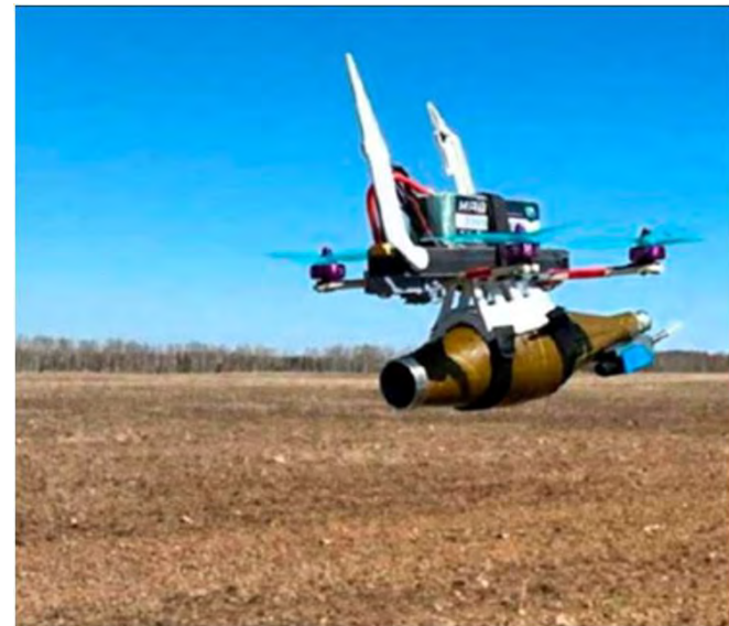
İPV kamikaze drone with a warhead based on an RPG-7 rocket
