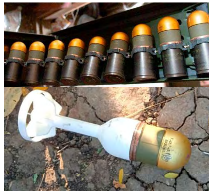
40x53 mm grenade (USA), adapted for deployment from UAVs
