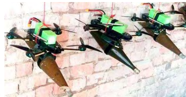
PG-7V warheads mounted on IPV drones
