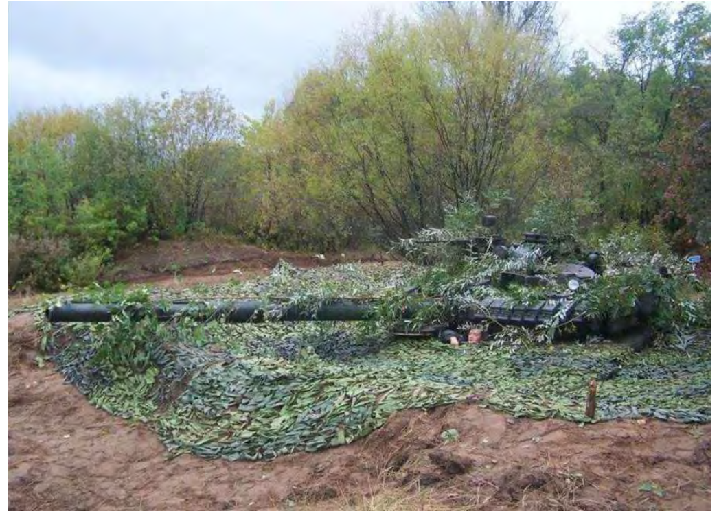
When installing camouflage nets on equipment, avoid geometrically regular shapes and strive for natural ones.
