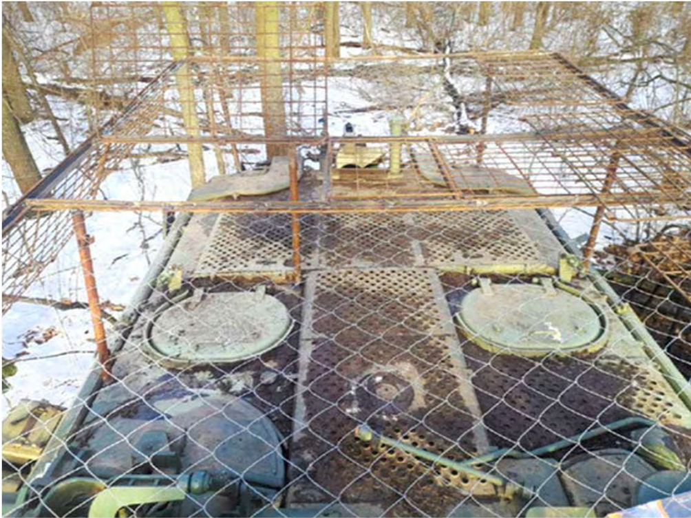
Protecting armored vehicles with chain-link fencing from drops and simple kamikaze drones
