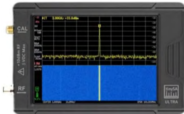
Tiny SA Ultra spectrum analyzer with special firmware "PEP UAV v2.5.2a"
