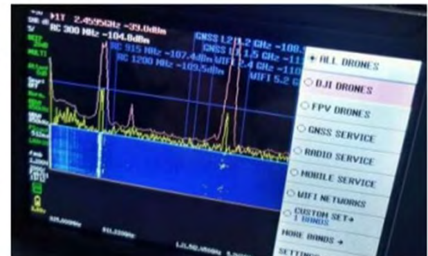
Tiny SA Ultra spectrum analyzer with special firmware "PEP UAV v2.5.2a"
