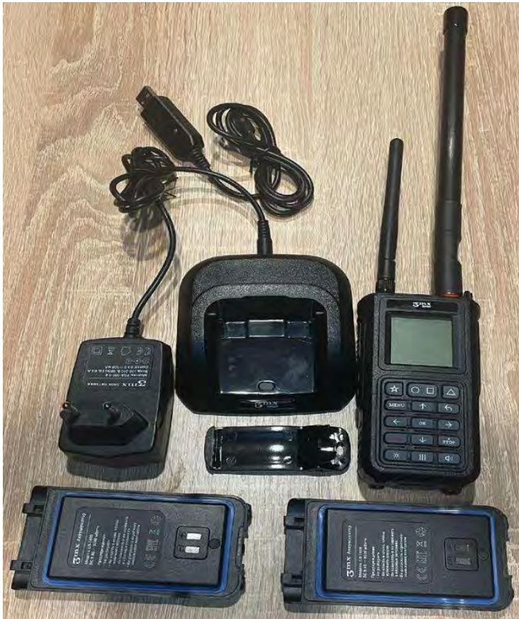
Omnidirectional UAV detector "Bulat" v.4 (manufactured by "3MX")
