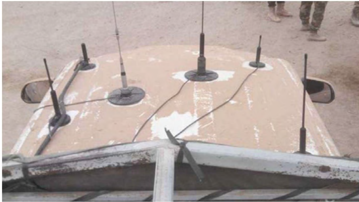
Placement of the Lesochek jamming station on the hood of a car
