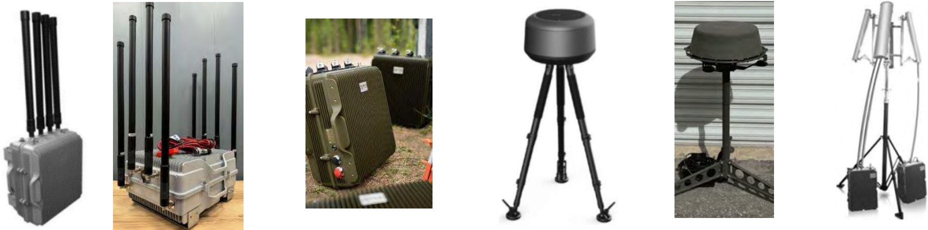
Examples of portable dome electronic warfare systems with circular and sector (panel) antennas
