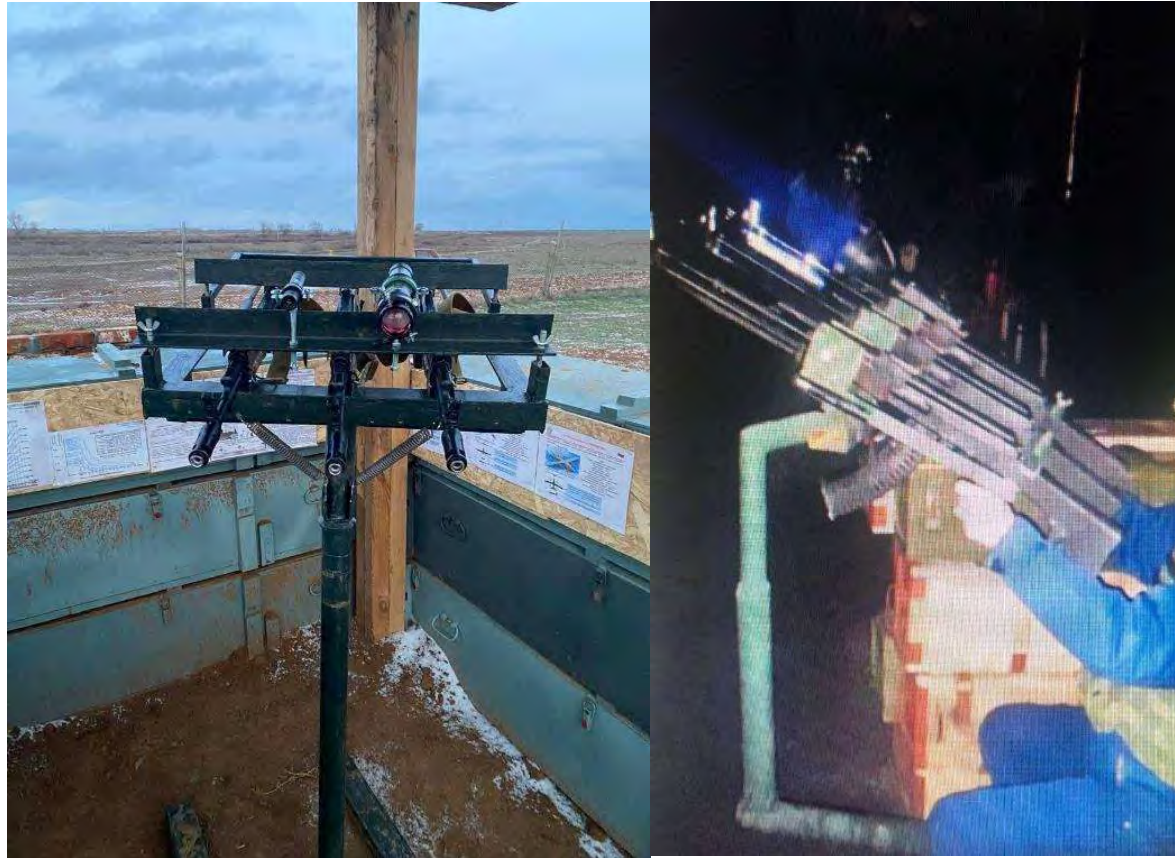
Left: a typical stationary PVN position, fortified, with memos on UAV types and fire control, a stationary installation of three AK-74M assault rifles Right: Use of paired assault rifles as stationary air defense
